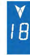
蓝底白字 16段码液晶显示 Blue background white character 16 segments LCD display
