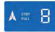
蓝底白字 16段码液晶显示 Blue background white character 16 segments LCD display
